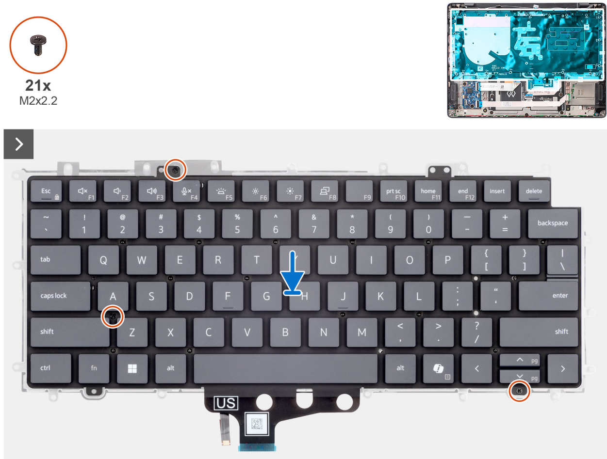
Figure 80. Installing the keyboard
